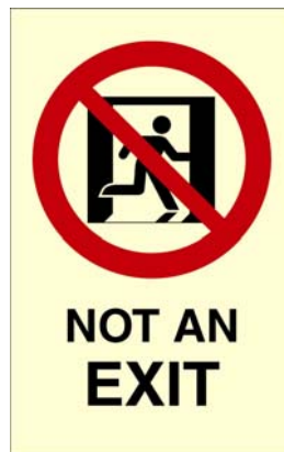
Exhibit 9 Sign for non-exit door using optional NFPA “no exit” symbol.
