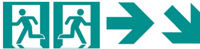
Exhibit 1. ISO 7010 Egress symbols E001 and E002, ISO 7010 Directional arrow E005 and E006.
