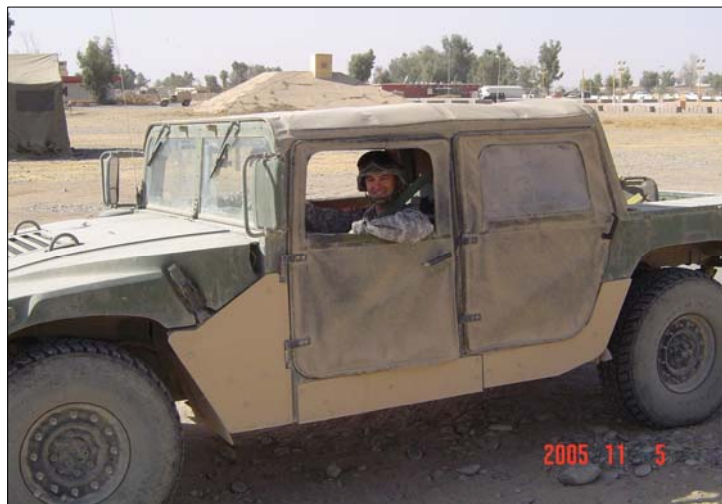
Exhibit 9: The canvas-covered M-998 HMMWV with “soft-skinned” top and sides provided little to no protection from insurgent IEDs, shrapnel and bullets.
