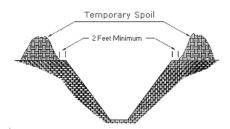
If possible, keep the grade away from the excavation. Provide scaling to remove loose rock or soil or install protective barricades and other equivalent protection to protect from the hazard of falling rock, soil or materials. Do not work on the faces of sloped or benched excavations at levels above other workers unless the workers at lower levels are adequately protected.
