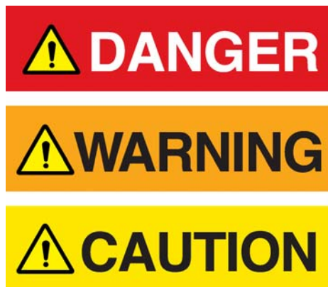
Exhibit 5. The signal word panel for ANSI Z535.2 safety signs using the ISO safety alert symbol
