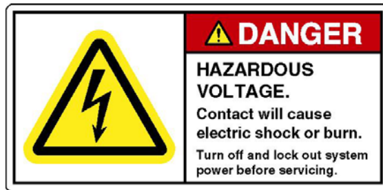
Exhibit 6. Example of an ANSI Z535.2 facility safety sign with ISO formatted symbol
