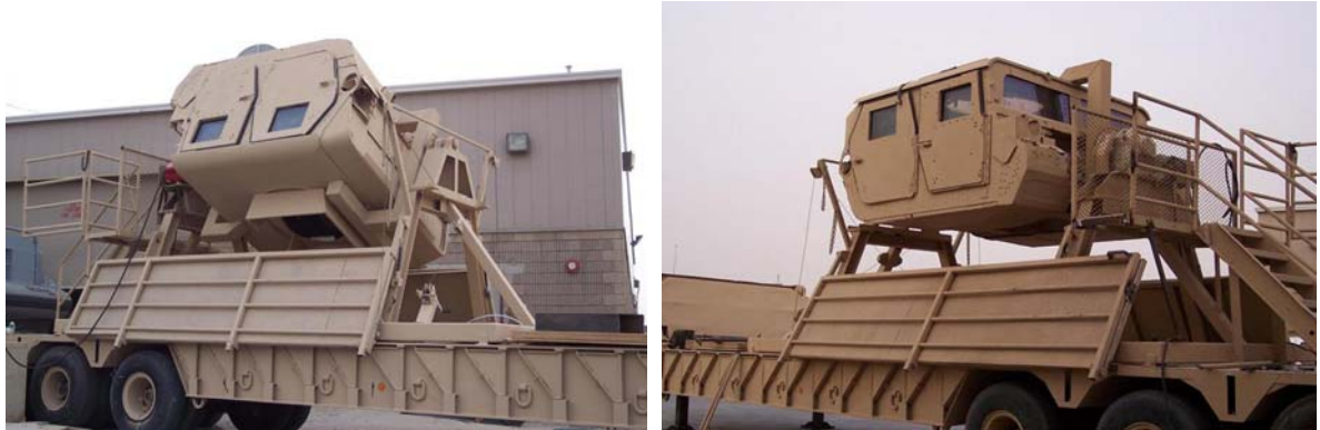
Exhibits 8 & 9: The trailer-mounted CFLCC version of the HEAT is fielded in Kuwait. Note the flip-down access platforms and safety guards.
