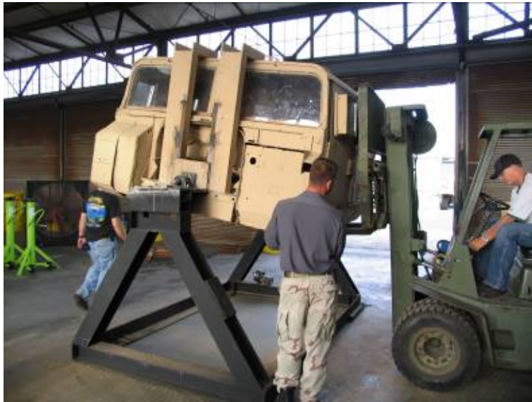
Exhibit 5: Jett, Hill and Whiting mounting the Humvee cab on the steel frame in an ECS 43 maintenance bay
