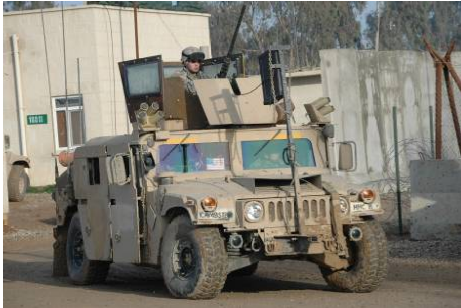
Exhibit 1: Adding protective armored plating and a turret raised the Humvee’s center of gravity and created an extremely top-heavy vehicle.
