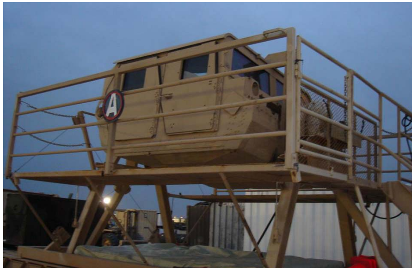
Exhibit 10: CFLCC HEAT access platforms and safety guards in position
