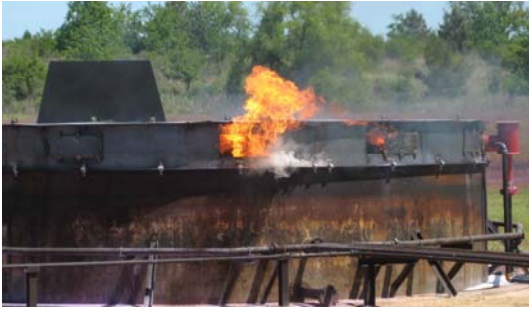
Exhibit 13 Test in IFR tank shows fire visible through both vent windows before being foamed.
