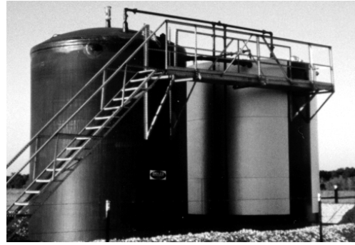
Exhibit 1. The diagram depicts a fixed roof tank such as the small fixed-roof E&P tanks on the right.
