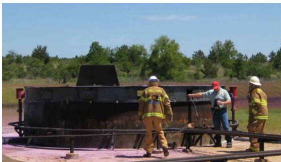
Exhibit 11 Crew is testing tank head space flammability.
