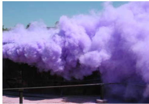
Exhibit 16 After foam leaves residual fires the phased application of vivid dry chemical flows from IFR tank vents.
