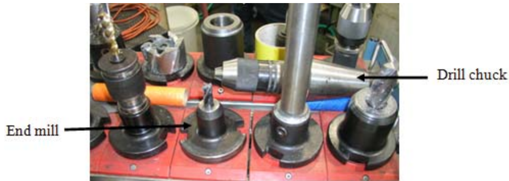
Figure 2. This is a tool holder with the drill chuck lying horizontally and out of place.
