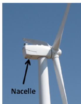
Figure 1: Wind Turbine Nacelle.
