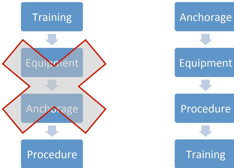
**Exhibit 1: This graphic compares a common, but incorrect, method for developing active fall protection systems with a correct practice.**
