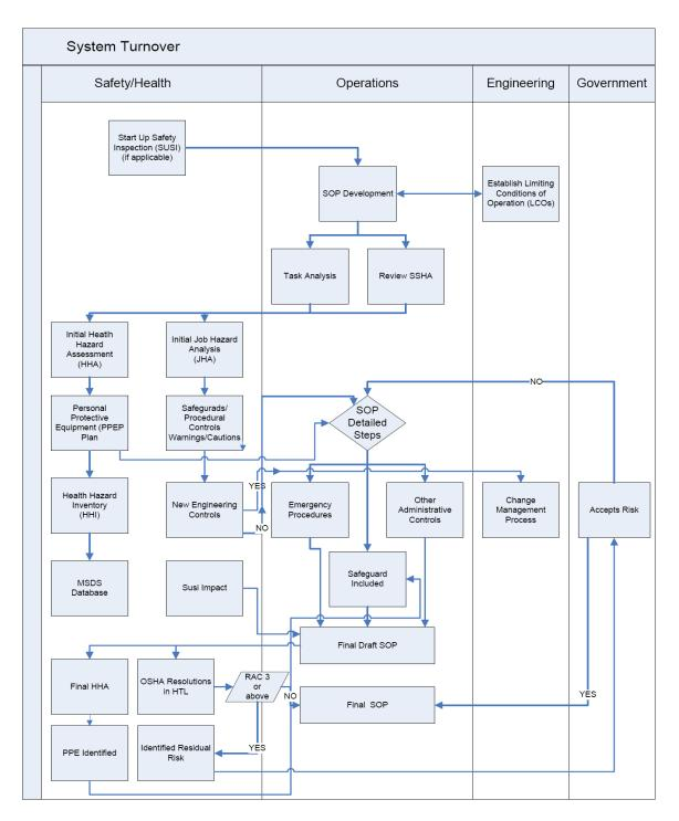
Exhibit 8. Block Flow Diagram for the development of procedures
