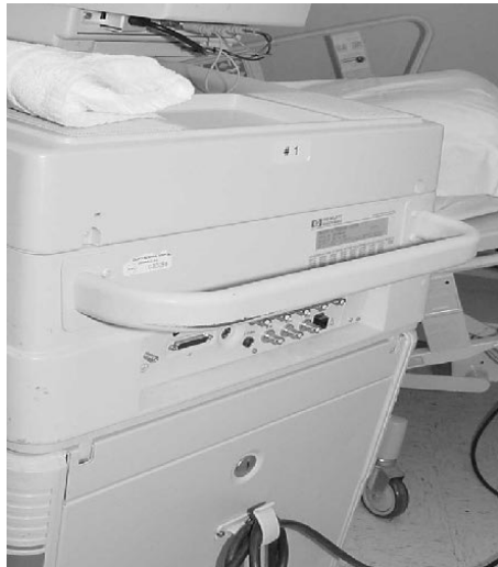
Photo 4a (before) and 4b (after): A foam grip was installed over the existing handle in order to provide a soft and compressible hand/handle interface when transporting the unit for portable studies.
