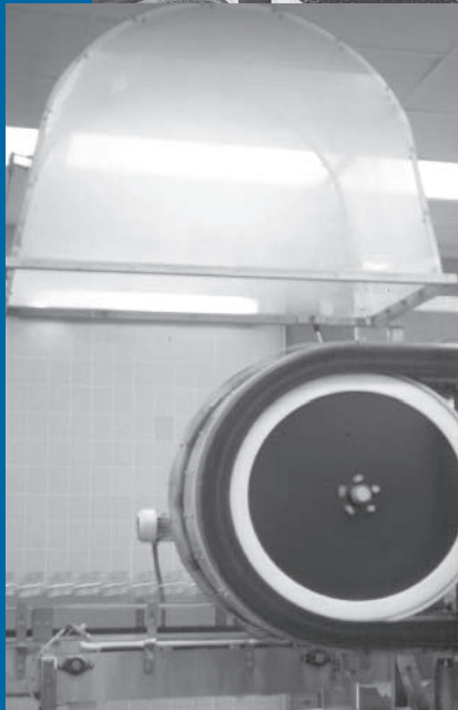
Clockwise from top: Devices such as pressure-sensitive mats (top) and interlocking guards (above, right; below, right) stop or prevent operation of machines to protect operators. In many cases, however, guards can be bypassed or removed (above), exposing the operator to the risk of serious injury.
