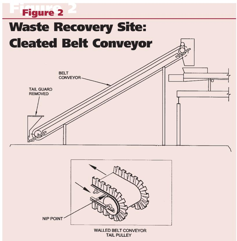
While realigning the unit, the maintenance worker discovered that he needed a part and went to retrieve it, leaving the tail take-up guard off. A foreperson (who was not involved in the realignment process) observed debris collecting at the tail pulley,
