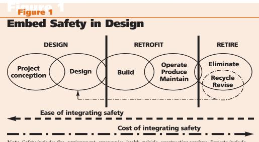
**Note.** Safety includes fire, environment, ergonomics, health, vehicle, construction workers. Projects include facilities, processes, equipment, products.
