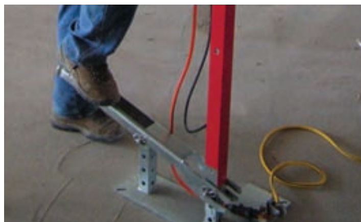
Photo 6 (top): Gravity pin for telescoping column of foot-lever drill press is visible at the top of the lower red column.
