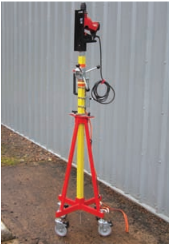
Photo 8 (above, left): A makeshift positive stop was added to prevent the drill bit from going too deep. The newer saddles have a built-in adjustable stop.
