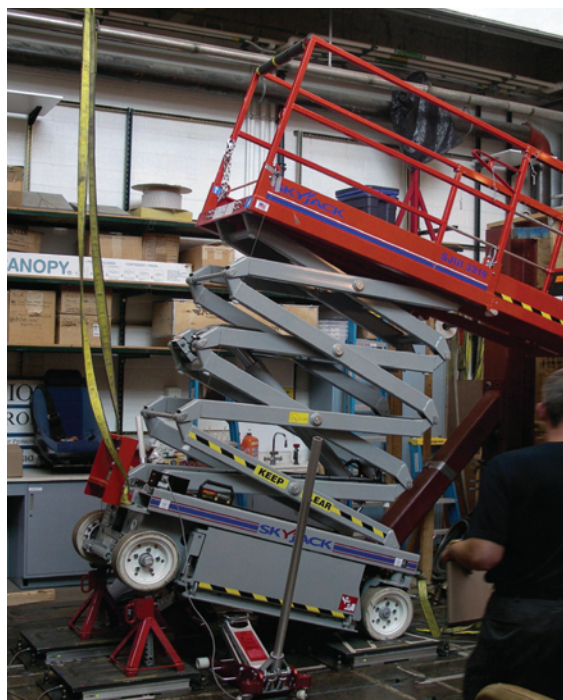
Photo 3 (above): To calculate CG in x and z directions (as shown in Figure 1), four force plates were placed under the wheels of the scissor lift.
