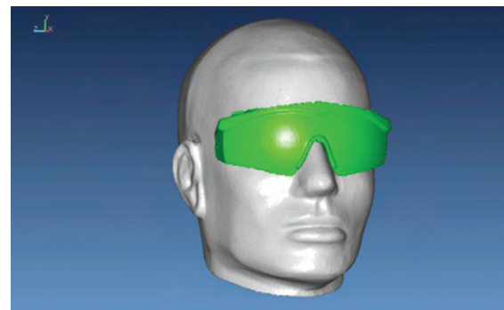
Photo 3: Example of eyewear scan digitally fit to headform scan for coverage coefficient calculations.
