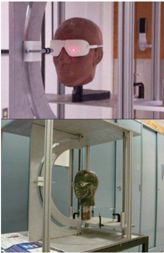
Photos 6 and 7: Physical coverage assessment test fixture.
