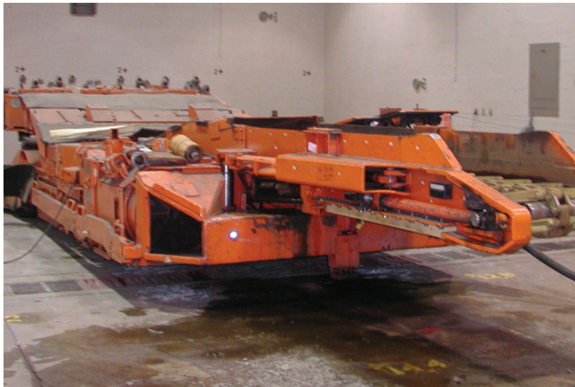
Photo 1: Operating large mobile equipment such as a continuous miner is one of the most dangerous jobs that workers perform in underground coal mining.
