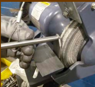
Photo 5: A safety gauge helps employees measure clearances easily and accurately.
