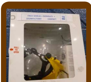
Photo 4: Storing a face shield, goggles/safety glasses, respiratory mask and disinfectant near the grinder helps workers comply with safe practices.
