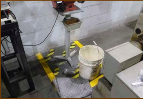
Photo 6: The permanent floor marking around the grinder can also quickly alert management to poor housekeeping practices that require correction.
