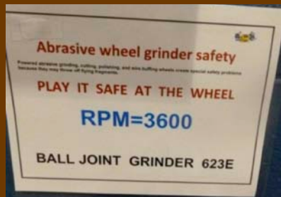
Photo 2 (left): Reading this grinder's RPM requires the worker to examine the device closely. Thus, it is best to conspicuously display this information (Photo 3, right) so that the operator can quickly compare grinder and wheel RPMs.
