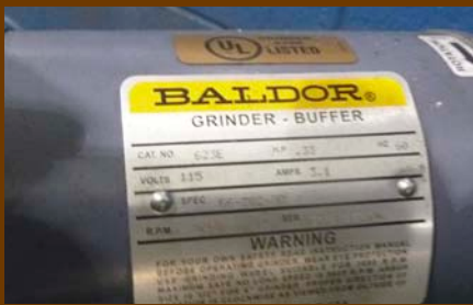
Photo 2 (left): Reading this grinder's RPM requires the worker to examine the device closely. Thus, it is best to conspicuously display this information (Photo 3, right) so that the operator can quickly compare grinder and wheel RPMs.
