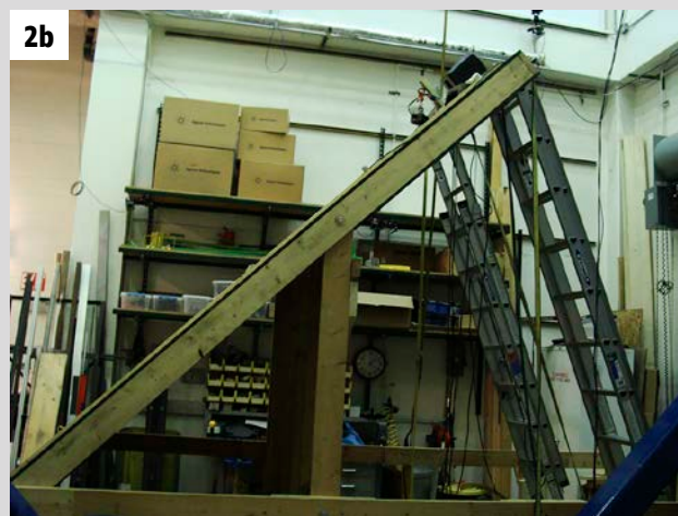
Figure 2b (left): Test roof configuration for the 8 in 12 (34°) slope. Figure 2b (right): Test roof configuration for the 12 in 12 (45°) slope.
