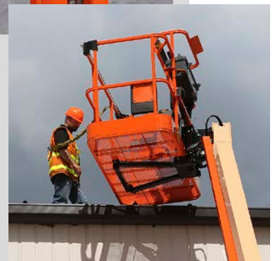
Photo 1 (above): An anchorage subsystem that allows for limited excursions outside of the MEWP, if jobsite or local restrictions allow.
