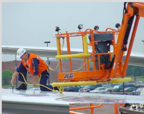
Photos 3 and 4 (above, right): The pictured aircraft external fall arrest anchorage subsystem allows one worker limited excursions outside of the MEWP, if the jobsite and local restrictions allow. Specific guidelines for use and inspections are in the operator's manual and must be followed.
