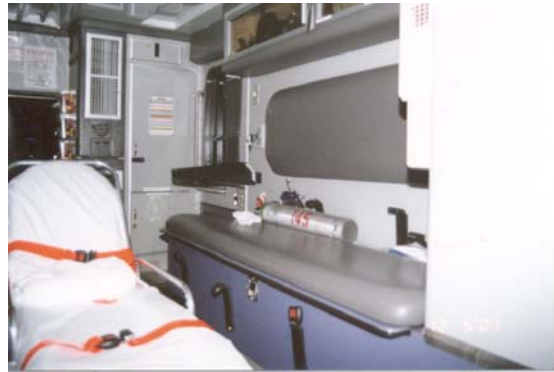
Exhibit 1. View from the rear looking forward to the right or curb side where a loose oxygen bottle sits on the bench and head impact risks from cabinets are present.
