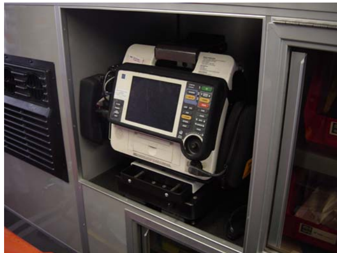
Exhibit 12. Hard mounted EKG unit to adjustable, sliding bracket installed in compartment to remove projectile risk associated with loose equipment while providing easy access for most workers.
