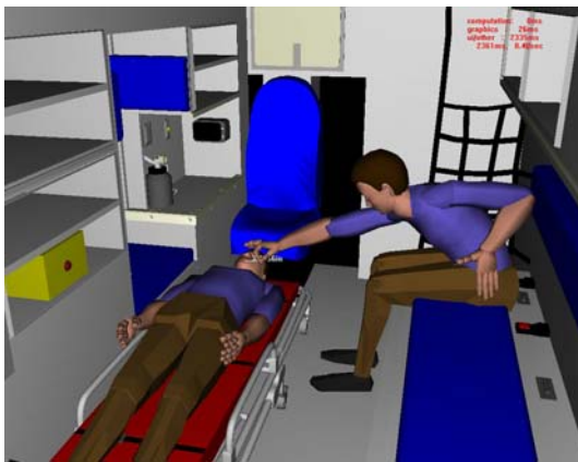
Exhibit 5. This image depicts a seated manikin, restrained at the hips as would be observed when using a required lap belt on the bench seat of a typical ambulance built to the GSA, KKK-1822 Star of Life (SOL) ambulance specification.
