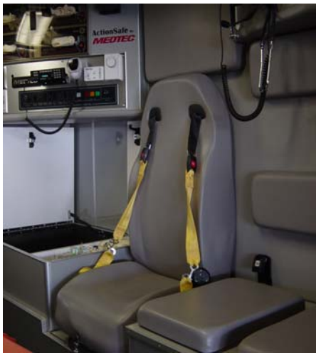
Exhibit 11. The angled communication cabinet, sliding seat with 5 pt harness, and removed overhead curb side cabinet are illustrated.
