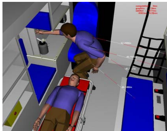
Exhibit 6. This image depicts a standing manikin, restrained at the hips and shoulders, but free to move as needed as would be observed when using a mobile restraint on the bench seat of a retrofitted, SOL specified, ambulance.
