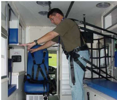
Exhibit 19. 50 th male demonstrating mobile restraint in the standard SOL ambulance while reaching for suction unit.
