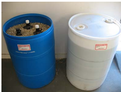
Exhibit 2. Comparison of a lab over-pack drum (left) versus a bulked drum of compatible waste (right).
