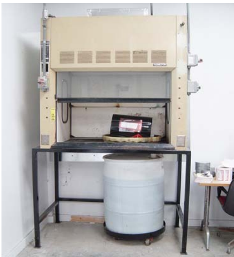
Exhibit 3. A picture of the modified fume hood in the UH hazardous waste facility.
