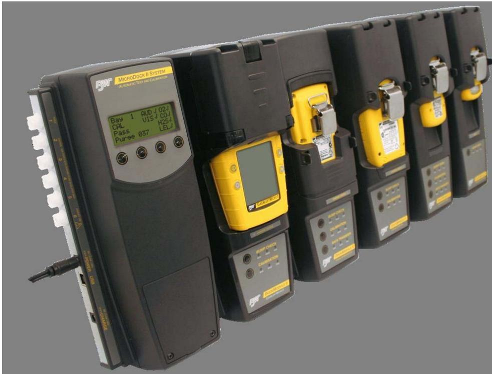
Increasing in popularity is the use of a docking station that will do the functional test, calibrate, record data and charge the monitors. In case of an event where evidence of proper maintenance and care of a gas detector must be given, docking stations provide objective proof that procedures are being followed.
