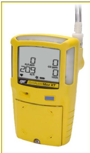
Today's gas monitoring equipment has come a long way from the miner's canary. Workers need to have a personal multi-gas monitor to perform the required atmospheric pre-testing and continuous monitoring. The monitor needs to be easy to use, rugged and reliable to work in some of the adverse conditions that can exist in these environments.
