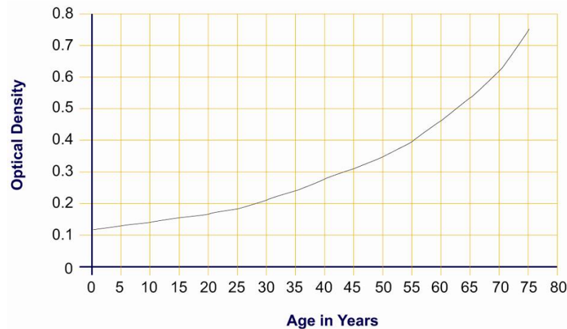
Figure 1: Loss of transmission of blue light (460nm) through the lens of the eye due to aging (Source: Meale, 1973)
