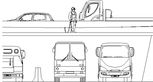
Figure 16. Worker will impact roadway before fall protection starts deceleration
