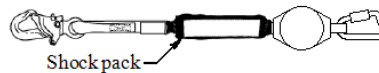
Figure 9. SRL with shock pack energy absorber, 2-ft free fall, only 2-ft payout
