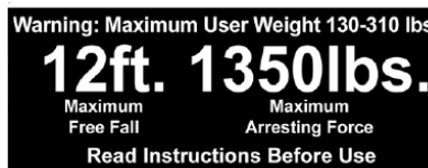
Figure 6. New 12-ft free fall label (limited to 6-ft free fall if user exceeds 310 lbs)
