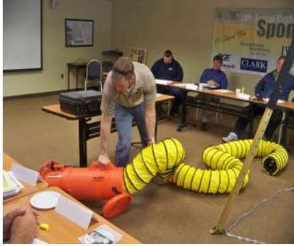
Exhibit 7. Ventilation blower and hose.
