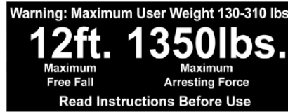
Figure 4. New 12-Foot Free Fall label clearly defines the maximum free fall limit to be 12 feet.
