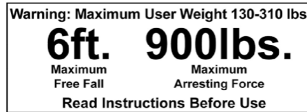
Figure 2. New 6-Foot Free Fall label clearly defines the maximum free fall limit.
