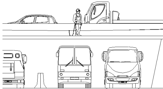
Figure 11. Worker will impact roadway before fall protection starts deceleration.
