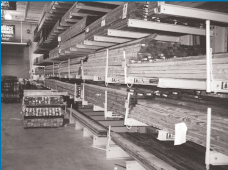
Photo #10 (above) shows lumber stored on cantilever racks. The retainer bars prevent the lumber from falling off the open sides.
