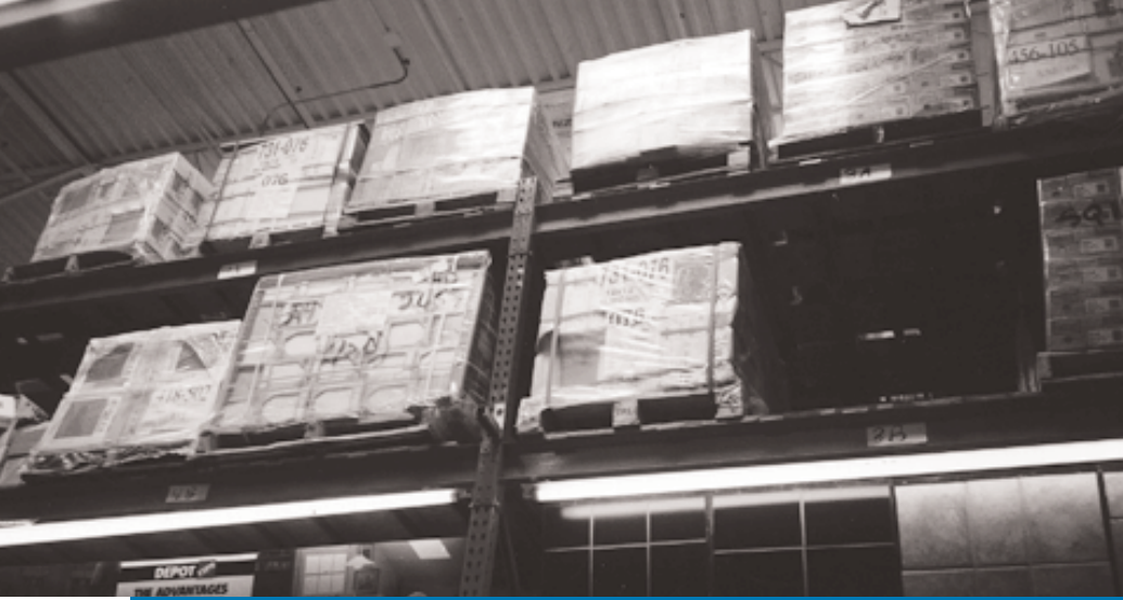
Photo #7 (left) shows several shrink-wrapped pallets on the pallet rack. The pallets are all even with the sides of the rack. Shrink-wrapping reduces the risk of a carton being knocked off the rack.
