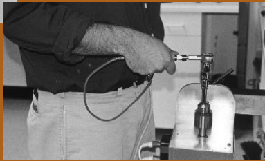
Photo 3 (clockwise from right): Screwdriver task apparatus. Photo 4: Ratchet task apparatus. Photo 5: Lift-and-carry task apparatus.
