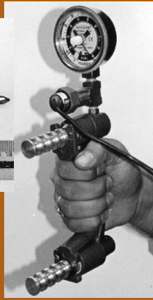
Photo 1 (far left): Experimental handle configured as a screwdriver. One handle segment is removed to reveal the instrumented core. Photo 2 (left): Hand dynamometer. A pressure transducer was inserted between the dynamometer body and dial gauge.
