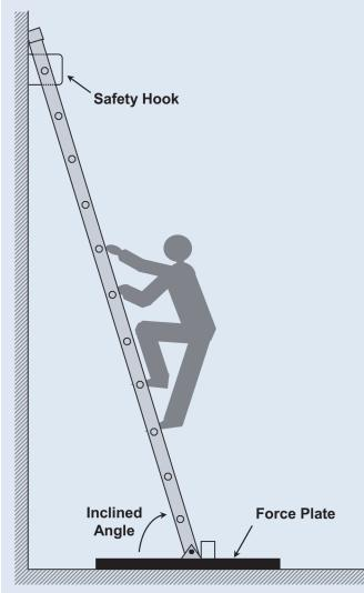
Abstract: The slipping of the bases of portable ladders away from the wall is a major cause of injuries. This article summarizes causes and potential interventions. These include developing practical guidelines on proper ladder setup and reminders not to rush on a ladder. In addition. users should know to avoid setting up ladders over contaminated areas, as well as to always use antislip ladder shoes.
