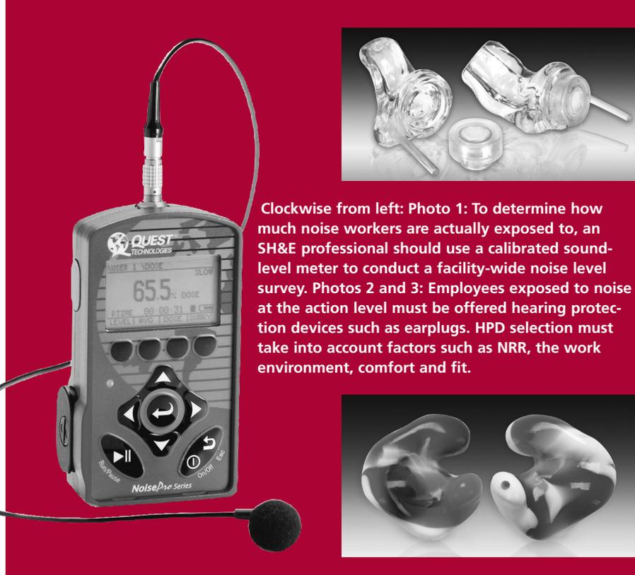
Clockwise from left: Photo 1: To determine how much noise workers are actually exposed to, an SH&E professional should use a calibrated sound-level meter to conduct a facility-wide noise level survey. Photos 2 and 3: Employees exposed to noise at the action level must be offered hearing protection devices such as earplugs. HPD selection must take into account factors such as NRR, the work environment, comfort and fit.
