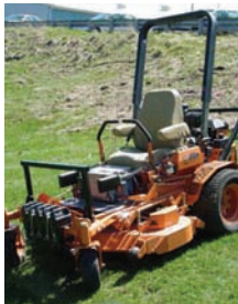
A telescoping AutoROPS offers tractor rollover protection while allowing the tractor to be operated in low-clearance settings (Photo 2, top) such as orchards and animal confinement buildings. AutoROPS can be used on farm tractors (Photo 3, center) and commercial lawn mowers (Photo 4, bottom).
