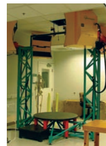
Photo 5: A Cyberware WB4 3-D full-body scanner was used to register the interface between human torsos and fall-arrest harnesses while the subject was in both the standing and suspended postures.
