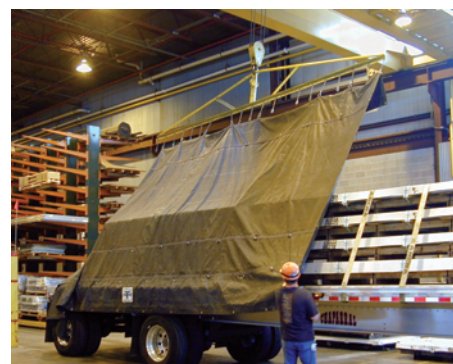
Photo 2 (above): The side kit is fitted and tied down with bungee cords to the flatbed.
