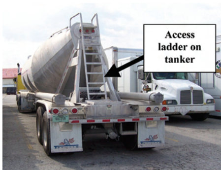
Photos 4 and 5 (from top): Tanker trucks usually have fixed ladders to help drivers access the top of the tank. Fall protection for the driver once s/he is atop the tank—at least 15 ft above the ground—is problematic.
