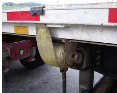
Photo 7: Tarp tie-downs are tightened and secured to the rub bar.
