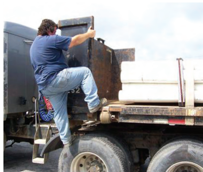
Photos 8, 9 and 10 (from top): If a flatbed truck is equipped with a header board across the front edge of the trailer, then it is more difficult for the driver to get onto the load from the platform behind the cab. The driver must either climb over a tire onto the bed or climb onto the rear of the truck bed using the ICC bar.
