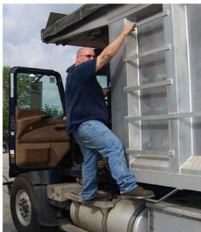
Photo 6: If a driver attempts to access the dump truck bed to clean it, when the tarping mechanism fails or for some other reason, s/he may be exposed to several hazards, including falls.
