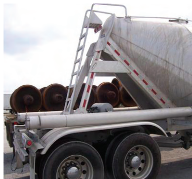
Photos 4 and 5 (from top): Tanker trucks usually have fixed ladders to help drivers access the top of the tank. Fall protection for the driver once s/he is atop the tank—at least 15 ft above the ground—is problematic.
