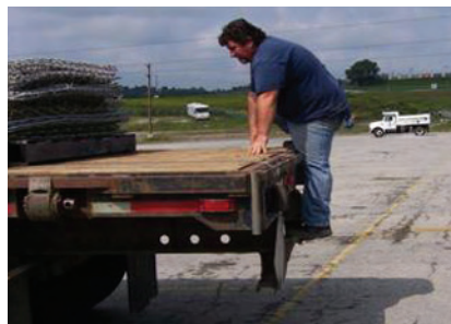
Photos 8, 9 and 10 (from top): If a flatbed truck is equipped with a header board across the front edge of the trailer, then it is more difficult for the driver to get onto the load from the platform behind the cab. The driver must either climb over a tire onto the bed or climb onto the rear of the truck bed using the ICC bar.
