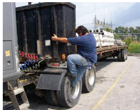
Photos 8, 9 and 10 (from top): If a flatbed truck is equipped with a header board across the front edge of the trailer, then it is more difficult for the driver to get onto the load from the platform behind the cab. The driver must either climb over a tire onto the bed or climb onto the rear of the truck bed using the ICC bar.
