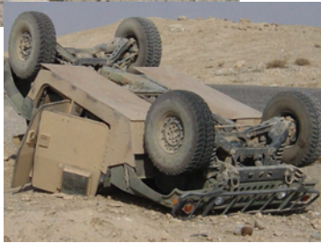
Photos 1 and 2: The unsecured soldier seated behind the driver was thrown out of the rear passenger door when it opened during the rollover.
