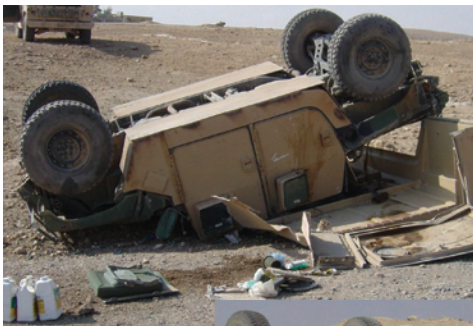
Photos 1 and 2: The unsecured soldier seated behind the driver was thrown out of the rear passenger door when it opened during the rollover.
