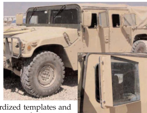
Photo 3 (top): The canvas-covered M-998 HMMWV with "soft-skinned" top and sides provides little protection from IEDs, shrapnel and bullets.
