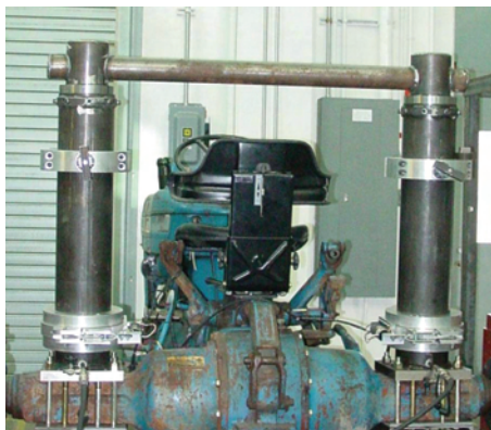
Photo 3: Second-generation AutoROPS on Ford 4600 in lab.
