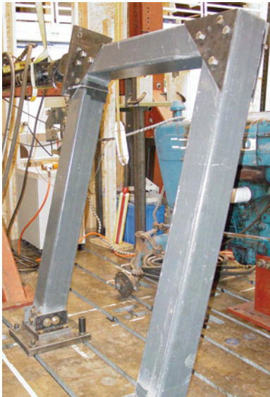
Photo 6 (left): Composite ROPS condition shown before static testing load was applied.
