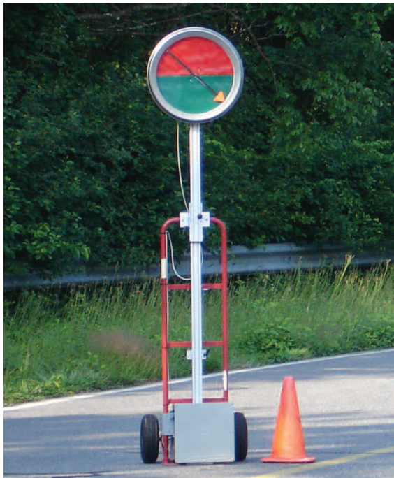
Photo 1: One of five pace clocks positioned around the test track. The bottom half of each pace clock face was green and the top half was red. An arrow hand moved around the pace clock at a constant rate and drivers were told to pass by the pace clock when the arrow was in the green portion of the clock face.
