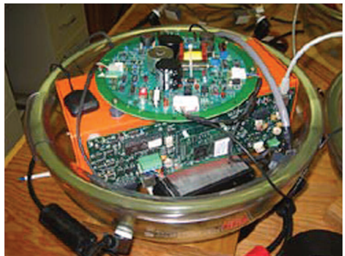
Photo 3 (a & b): Two opened glass spheres, one with primary lithium batteries (left) and one with electronics (right).
