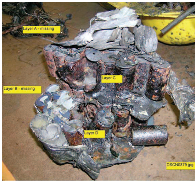
Photo 5 (left) shows an undamaged battery pack, where layers A-D represent the various lithium battery cell layers that make up the battery pack. Photo 6 (right) shows a damaged primary lithium battery pack after fire and explosion in OBS.
