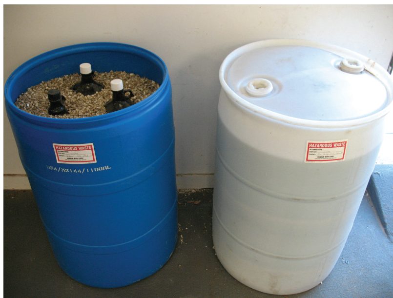
Photo 1: Comparison of a lab over-pack drum (left) versus a bulked drum of compatible waste (right).
