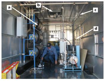
Photo 6: Missouri S&T's mobile hydrogen unit showing a) compressed hydrogen tanks; b) ventilation system; c) warning light; and d) emergency shutoff button. Not visible in this picture are hydrogen sensors and another emergency shutoff device located on the outside of the trailer. centered cubic crystal structure, such as iron and tungsten, should be avoided whenever practical. Cast iron shall not be used.
