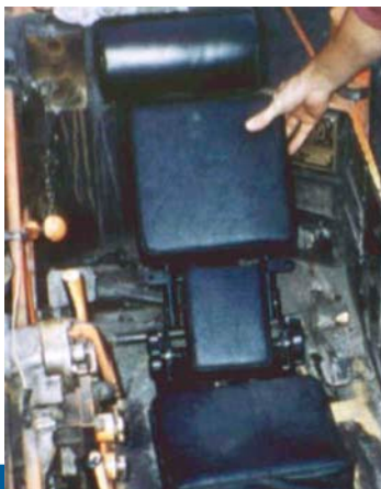
Photo 2 (a, top): Existing design for low-seam shuttle car seat; and (b, bottom) NIOSH's experimental design.
