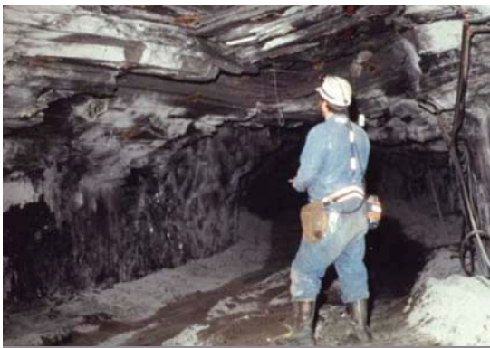
Photo 2: Initiation of roof cutter in a coal mine.
