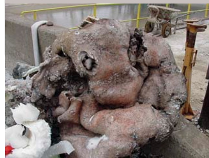
Photo 2: Combustible solid removed from the tank.
