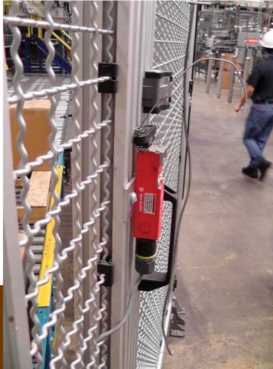
Photos 1 and 2 show an access door controlled by an interlock switch with broken cable.
