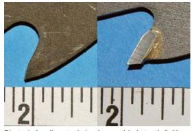
Photo 1: An alloy steel circular saw blade tooth (left) looks different from a carbide tooth tip (right).
