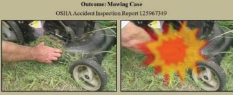
With the engine running, a worker used his hand to remove grass from a clogged lawn mower.
