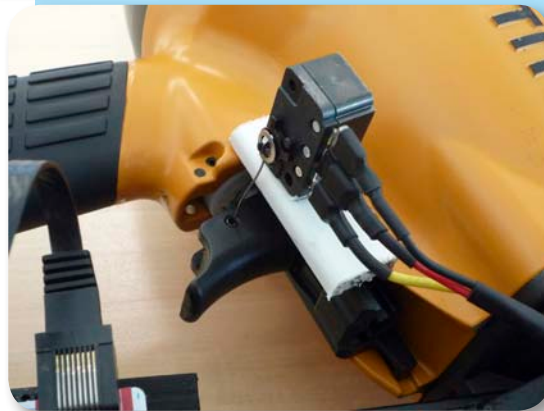
Photo 6 (bottom): Discharge controller on trigger actuates fastener discharge when trigger is pulled. The servomotor is connected to the trigger by a thin metal rod (through a hole in the trigger). When activated, the servomotor pushes the rod against a button inside the trigger that allows the piston cylinder to discharge a fastener.
