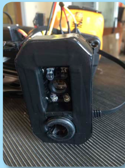
Side (Photo 4, left) and bottom (Photo 5, right) views of the nosepiece light sensor. Four LEDs illuminate the substrate for the light sensor to measure its RGBW light levels. A black enclosure (Photo 5) surrounds LEDs and sensor to protect them and minimize effects of ambient light.
