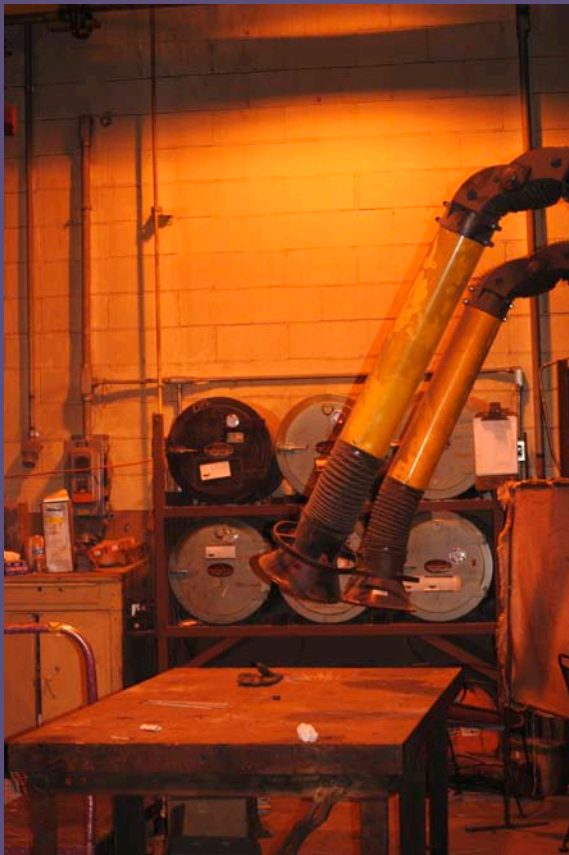
Photos 4 and 5: Welding ventilation (Photo 4, above) is essential to combat possible chemical exposure hazards found in many weld shops (Photo 5, left).
