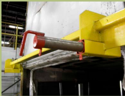
(Clockwise from top): Mechanical pin control for press (gravity energy control); lock-out of electrical plug; lockout performed on gate entry (alternative method); tagout; safety block for a press; group lockout; local lockout control.
