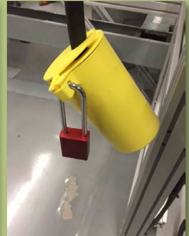
(Clockwise from top): Mechanical pin control for press (gravity energy control); lock-out of electrical plug; lockout performed on gate entry (alternative method); tagout; safety block for a press; group lockout; local lockout control.
